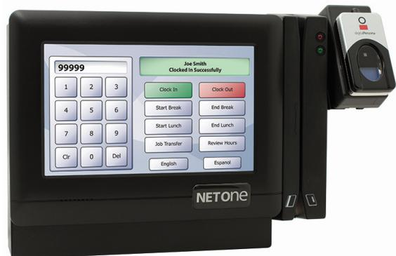
The NETOne cloud clock is a sophisticated data collection device that pushes punches to Vista Time as they occur. Employees can also use the touchscreen interface to perform self-service functions at the terminal. It recognizes swipe card or fingerprint reading, depending on its configuration.
